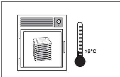
**1** Store the unopened pouches of plates at frozen or refrigerated temperatures  $\leq 8^{\circ}\text{C}$  ( $\leq 46^{\circ}\text{F}$ ). Use before expiration date on package. It is best to allow pouches to reach room temperature before opening.
