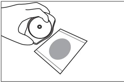
**7** Remove the spreader and leave the plate undisturbed for one minute to permit the gel to form.
