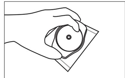
**6** Press firmly on the center of the spreader to distribute the sample evenly. Spread the inoculum over the growth area before the gel is formed. Do not slide the spreader across the top film.
