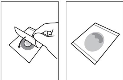
**4** Roll the top film down onto sample gently to prevent pushing sample off film and to avoid entrapping air bubbles. Do not let top film drop.
