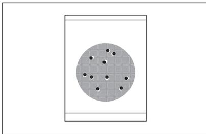
**9** 3M Petrifilm *E. coli*/Coliform Count Plates can be counted using the 3M™ Petrifilm™ Plate Reader, on a standard colony counter or other illuminated magnifier. Colonies may be isolated for further identification. Lift top film and pick the colony from the gel.
