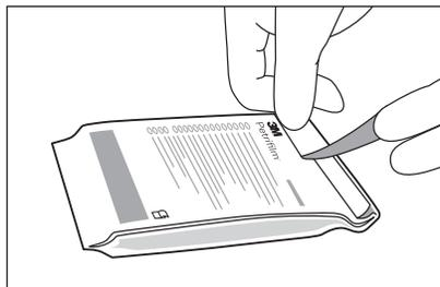
**2** Seal by folding the end of the pouch over and applying adhesive tape. **To prevent exposure to moisture, do not refrigerate opened pouches.** Store sealed pouches in a cool dry place for no longer than four weeks.
