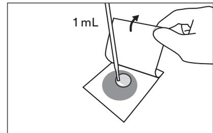
**3** Place 3M Petrifilm *E. coli*/Coliform Count Plate on flat, level surface. Lift the top film and with a 3M™ Electronic Pipettor or equivalent held perpendicular to plate, dispense 1 mL of sample suspension onto center of bottom film.
