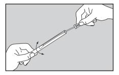
8 Wring out the contents of the swab tip by pressing and twisting the swab against the wall of the tube.
