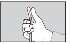
2 At the sampling location, prepare the swab by holding it with the bulb end near your thumb. Bend the red snap valve at a 45° angle until you hear the valve break. This allows the letheen broth to flow into the tube end and wet the swab.
