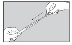
6 After sampling is complete, securely insert the swab back into the swab tube and transport to the lab for inoculation. Plate the letheen broth swab solution as soon as possible. Go to step 7 of the Inoculation Methods Section.
