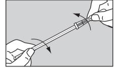
4 Twist and pull apart the bulb end of the swab from the tube end of the swab which contains the letheen broth.
