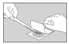
9 Carefully pour the entire contents of the tube onto a 3M<sup>™</sup>Petrifilm<sup>™</sup> plate. Follow current industry standards for disposal.
