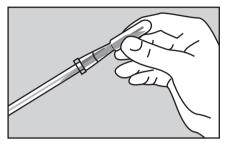
3 Squeeze the bulb of the swab to transfer all of the letheen broth to the tube end of the swab.
