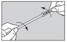
2 Twist and pull apart the tube end of the swab from the bulb end of the swab which contains the letheen broth.
