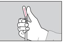
5 Prepare the swab by holding it with the bulb end near your thumb. Bend the red snap valve, at a 45° angle until you hear the valve break. This allows the letheen broth to flow into the tube end and wet the swab.
