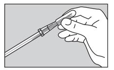
Squeeze the bulb of the swab to transfer all of the letheen broth into the tube end of the swab. Go to step 7 of the Inoculation Methods Section. Plate the letheen broth swab solution as soon as possible.
