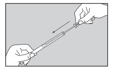
After sampling is complete, securely insert the swab back into the swab tube and transport to the lab for inoculation.
