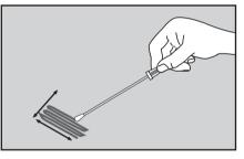
5 Hold the swab handle to make a 30°angle with the surface. Rub the swab slowly and thoroughly over the desired surface area. Rub the swab three times over this surface, reversing direction between alternating strokes.
