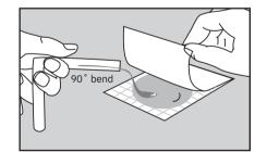
Use your thumb to bend the swab tube at a 90° angle at the highest mark that has diluent above it. Pour off a 1mL aliquot onto a Petrifilm plate. Repeat until the entire sample is used. Follow current industry standards for disposal. Refer to Petrifilm plate product package inserts for proper incubation and interpretation instructions.
