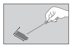
3 Hold the swab handle to make a 30°angle with the surface. Rub the swab slowly and thoroughly over desired surface area. Rub the swab three times over this surface, reversing direction between alternating strokes.
